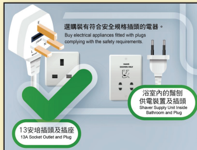
Plugs complying with the applicable safety standards of Hong Kong
