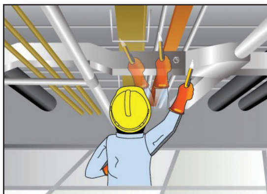
■ Testing whether the false ceiling is live
