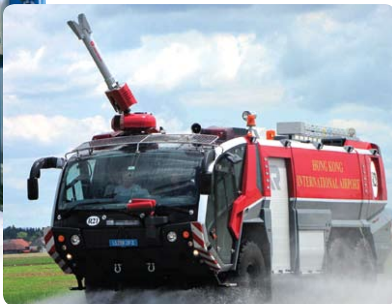
本部替消防處採購的快速截擊車，能讓該處在極短時間內撲滅因飛機事故引發之火警。 The procurement of the Rapid Intervention Vehicle by the Division allows the Fire Services Department to extinguish fire resulted from aircraft accident within a very short period of time.
